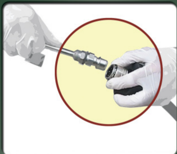
Connect twin hose assembly to end of each probe
