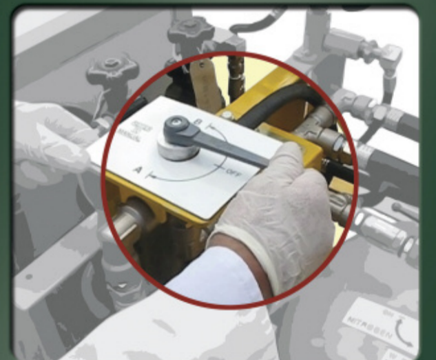
Refer to wash probe list and choose hose position A or B
