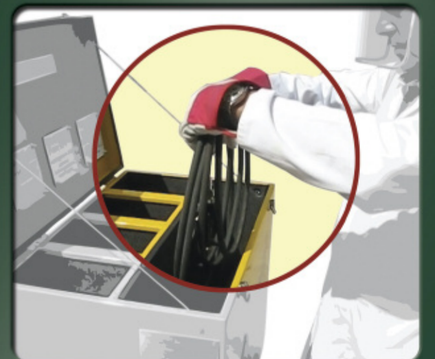
Disconnect blow-off hose and re-stow on the rig
