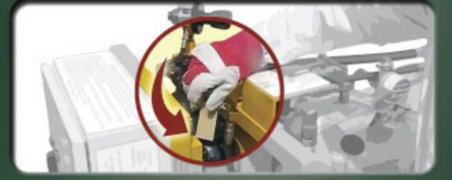
Open rig's nitrogen cylinders and, using donor regulator, charge in 250psi stages to a maximum pressure of 2500psi
