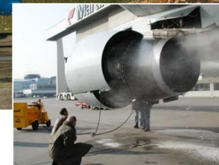
Air Europa following a simultaneous compressor wash of one engine of a Boeing 737 classic and one engine of a Boeing 737 new generation in Palma, Mallorca.
