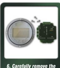
6. Carefully remove the PCB and set it face down on a soft cloth
