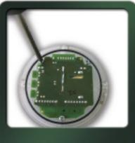
5. Unscrew the three **PCB** retaining screws
