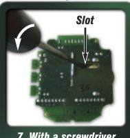
7. With a screwdriver lever the battery out through the slot in the PCB
