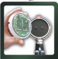
4. Carefully remove electronic module keeping rubber 'O' ring in place
