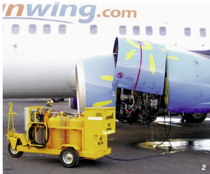
1 The 2x25 gallon rig, showing the tooling storage box to the rear, washing a Trent 772 engine fitted to an Airbus A330 for Corsair at Orly Airport, Paris
