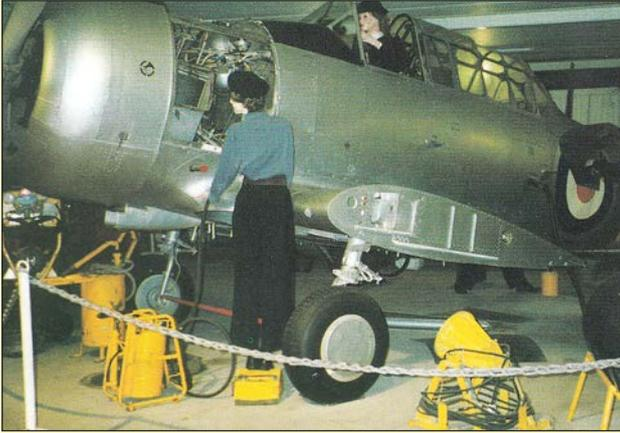
Juniper joined the Wrens in much of their important work keeping the fleet's pilots airborne. Here a Wren is depicted feeding engine oil into a Harvard trainer using one of our Mk2 rigs at the Fleet Air Arm Museum at the Royal Naval Air Station at Yeovilton.
