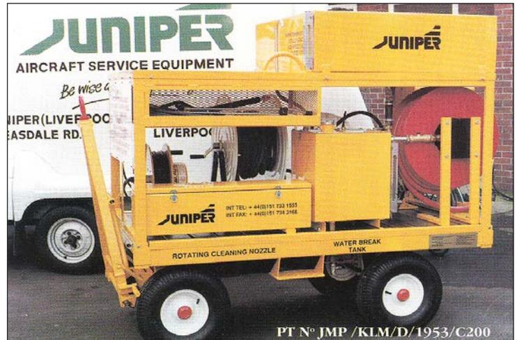
An extra 65 gallon water tank on the Juniper Aircraft Vacuum Toilet Cleaning Rig (JMP/KLM/D/1953/C500) has made it much more user friendly. Britannia are currently using the rig on their fleet of Boeing 767s at London Luton Airport. Boeing themselves have named us as a supplier of this rig in a recent service bulletin.
