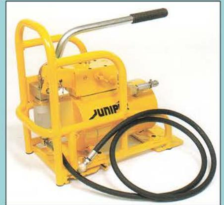
Our handy lightweight purging rig (JMP/HYD/D/4195) has been further developed into a handy hydraulic rig. Twelve units were purchased by the Royal Netherlands Navy to enable them to charge the Lynx helicopter oleo legs on board their frigates.
