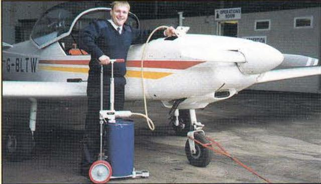
Angus Whyte from CATS topping up the engine oil on a Slingsby T67B Firefly aircraft with the new Risbridger unit.
