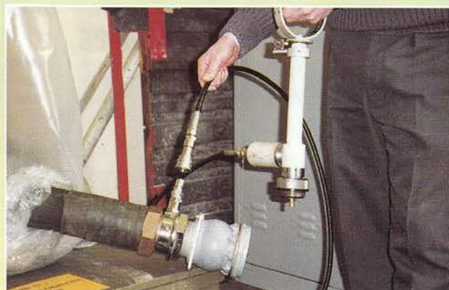
Unblended fuel, obtained at out of town locations can cause serious corrosion problems. To solve this problem, the RAF have utilised a Risbridger Oil gun and connected it to the refuelling hose with an adapter supplied with the Risbridger kit. This enables measured quantities of AL38 Fuel System Icing Inhibitor to be blended with the fuel as refuelling takes place.
