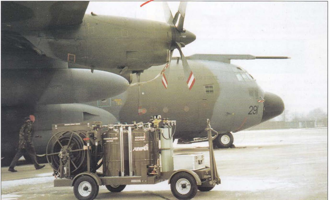
*An additional tank is required for a distilled water flush when turbine compressor washing the Hercules*
