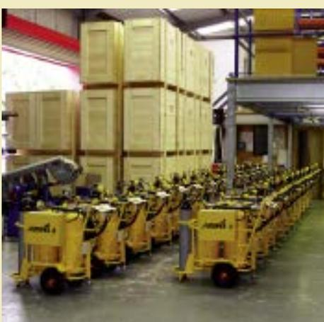
Completed mobile compressor washing rigs at our Ash House factory after the final check awaiting packing and despatch.
