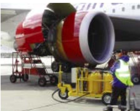
In May 2006 Virgin Atlantic Airlines invited Juniper to demonstrate the 2 x 25 gallon compressor washing rig performing a water wash on a CF6-80C2 engine fitted to one of their Boeing 747-400 fleet at Gatwick Airport.
