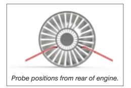
Guide the probes through the fan outlet guide vanes (ogv's) from the aft end, at approximately the **4 & 8 o'clock** positions, aft looking forward. Carefully from the aft end locate each tip so that they point between the booster inlet guide vanes into the booster and attach clamps. (See STEP 3 for clamping instructions).
