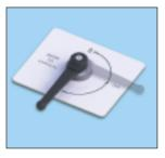
When using Passport engine wash probes, turn the three way selector to position '**A**' this ensures selection of the  $\frac{3}{4}$ " bore delivery hose.
