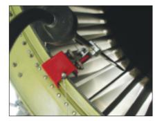
Guide the probe tube through the closest outlet guide vanes in relation to the clamping bracket and hook the 'J' hook nozzle of the probe over the Fan/Booster splitter with the tip aiming between the inlet guide vanes and into the engine core.
