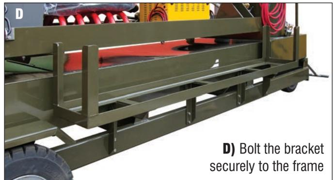
**D)** Bolt the bracket securely to the frame
