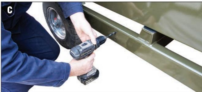
**C)** Drill the marked holes through the box section with 10mm clearance for the supplied fixing bolts (6 in total).
