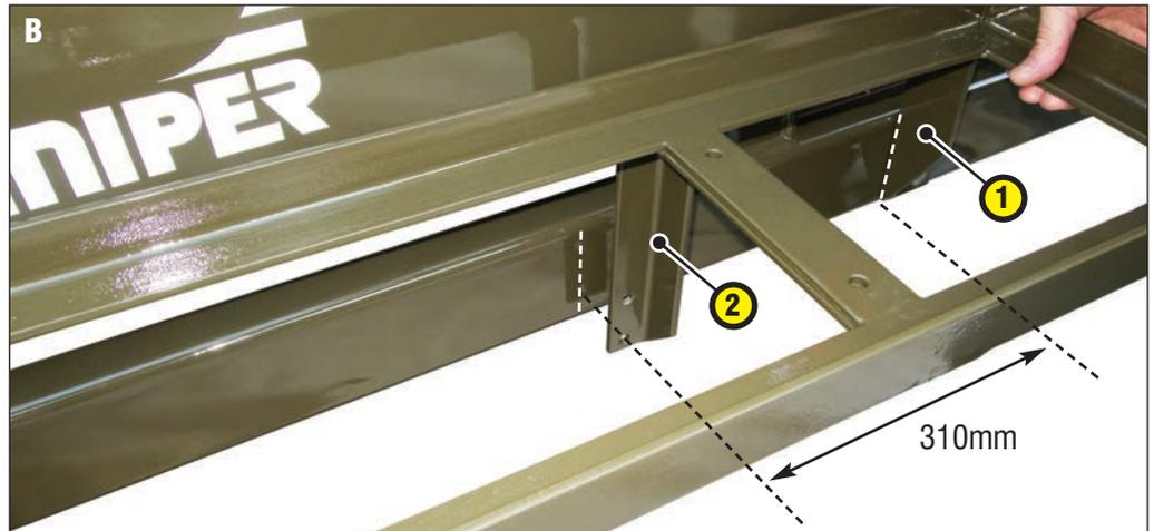
**B)** Measure 310mm in from the front vertical frame support (1) and mark a vertical line. With someone supporting either end of the bracket, align the pre-drilled holes in the first bracket mounting arm (2) with the vertical mark and mark the first two drill holes (the top one approximately 30mm down from the top of the frame section).
