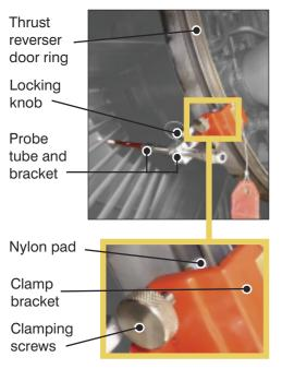
**CAUTION:** Ensure that the engine fan is held securely during fitting of the engine 'j' hook probes.
