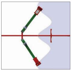
Position the probe clamps on the chevrons as shown above
