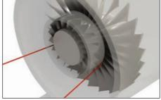
Guide the probes through the fan outlet guide vanes (ogv's) from the aft end, at approximately the **3.00 & 9.00 o'clock** positions, aft looking forward.
