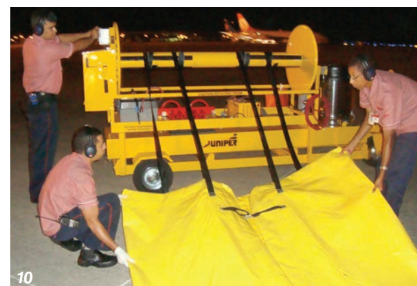
9 The Containment Mat in position during a recent engine wash for Aegean Airlines on a V2500 engine fitted to one of their Airbus A320 aircraft. The flexible vacuum hose is connected and ready for use.
