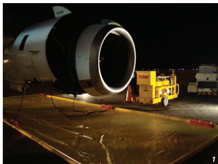
1 Juniper's 2x25 gallon wash rig (JMP/CFM56/D/4777/C200) in the livery of TAM Linhas Aereas being used with the new Containment Mat to wash the V2500 engine fitted to an Airbus A320 at the Jardim Aeroporto, San Paulo, Brazil in February 2010
