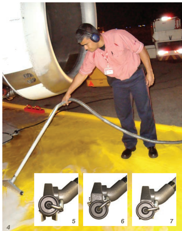
1 Juniper's 2x25 gallon wash rig (JMP/CFM56/D/4777/C200) in the livery of TAM Linhas Aereas being used with the new Containment Mat to wash the V2500 engine fitted to an Airbus A320 at the Jardim Aeroporto, San Paulo, Brazil in February 2010
